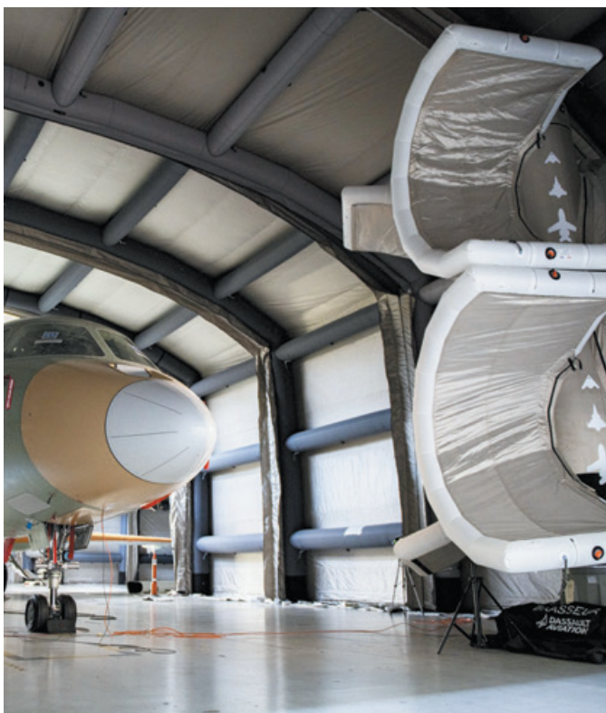
Inflatable Faraday cage developed by AirCaptif, in partnership with Dassault Aviation.
